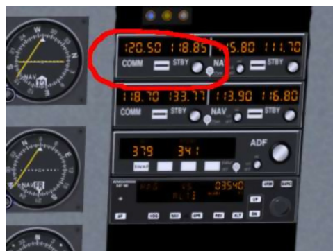
Figure 9.4: The C172 communications stack with COMM1 highlighted
