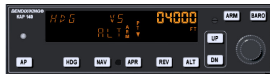
Figure 10.9: Autopilot with altitude armed
